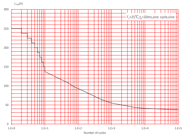
FIG.5: Non-repetitive surge peak on-state current for a sinusoidal pulse with width t_p < 20ms , and corresponding value of I^2t ( di/dt < 100A/\mu s )
